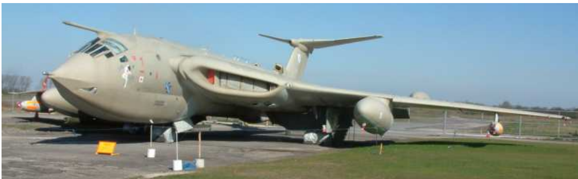
Victor XL231 ('Lusty Lindy') at the Yorkshire Air Museum, Elvington Originally a bomber, converted to an air-to-air refuelling tanker (refuelling pods far left and right)
